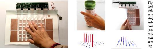
Figure 1. The PrintSense technique supports the development of multi-modal sensing arrays, printed as a single layer onto a flexible substrate and connected to a custom hardware module (left). It supports capacitive touch and proximity sensing along with resistive pressure sensing (centre) & bend sensing of the substrate (right).
