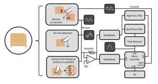
Figure 2. Three different signal detection schemes supported by PrintSense's inter-digitated electrodes. From top to bottom: active transmit-and-receive capacitive sensing for proximity and folding detection, AC hum detection for touch and proximity detection, and resistive pressure sensing.
