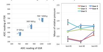
Figure 3. Left: Raw GSR and FSR ADC data from "tapping" (0~200 g), "pressing gently" (300~600 g) and "pressing hard" (700~1000 g). Right: Mean values of the GSR/FSR ratio for each user across time.
